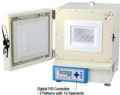
Digital Muffle Furnaces are well-built with digital PID control system, patented jog-shuttle control system and digital LCD with back-light function. The 4-side heating mechanism ensure the short heat-up time and high temperature uniformity, and the maximum temperatures are 1,000°C for FPX model and 1,200°C for FHX model.
