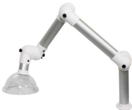
The flexible arm system of suction arms use friction joints and ball bearing for necessary grip and easy movement. Suction Arms can be fixed on wall/ceiling/worktop with adjustable arms and suction cup.
